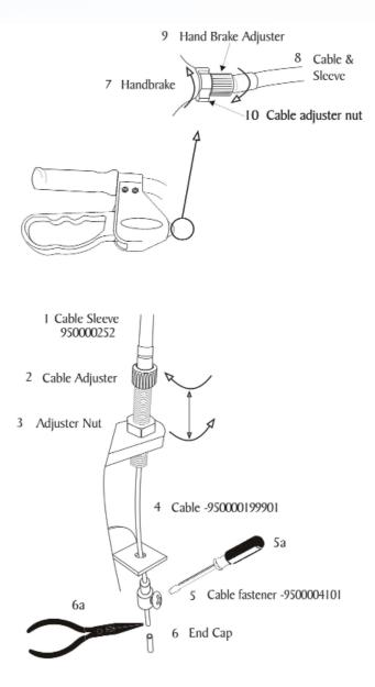
For minor adjustment, the brake adjuster (9) located on the handbrake (7) can be turned out from the handbrake counter clockwise to tighten the brake, or clockwise to loosen the brake. Keep the cable adjuster nut (10) against the handrail.
